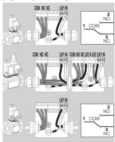
Double solenoid valve: if a plug with socket is fitted, only one proof of closure switch can be connected.
