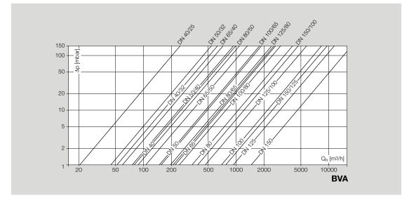
Butterfly valves for air and flue gas BVH, BVHR, BVHS, BVHM
