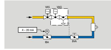
In pneumatic ratio control systems, the butterfly valve with mounted actuator IBA determines the air volume for the required burner capacity.
