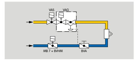
Solenoid actuator MB 7 and butterfly valve  $\mathsf{BVHM}$  are used for intermittent switching of the burner.
