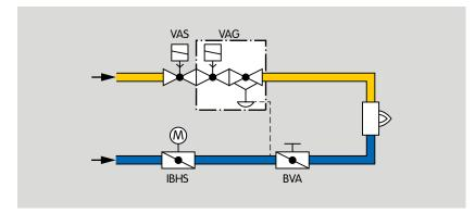
The safety closing function ensures that in the event of a mains voltage failure air cannot stream into the furnace without being under control.
