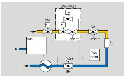
The butterfly valve with actuator IBH is used on burners that are operated with preheated combustion air at temperatures of up to  $450^{\circ}$ C ( $840^{\circ}$ F).
