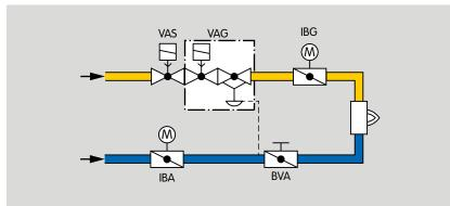
If the burner is to be operated with excess gas or air for reasons of process operation, the butterfly valve with actuator IBG can be used to correct the lambda value.
