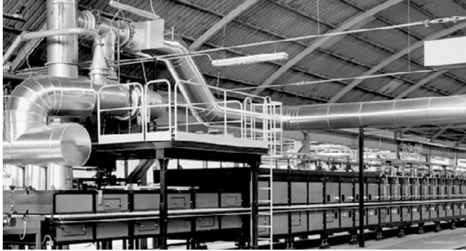
Roller hearth kiln in the ceramics industry
