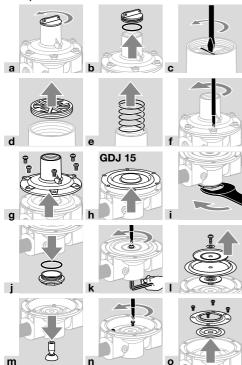
**P** Replace all diaphragms and sealing elements, except the valve seat.
