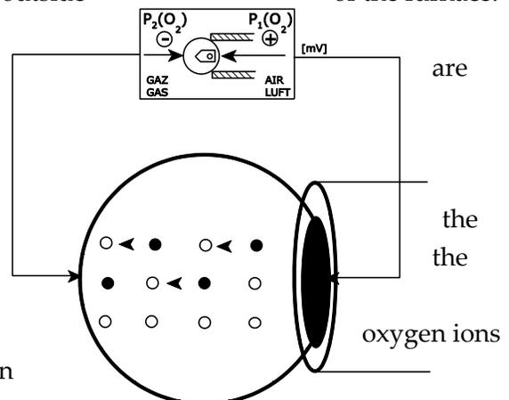
expression of the relations between the relative difference in oxygen concentrations between the ambient air and atmosphere in the furnace as well as the temperature of the sensor. Therefore, the voltage in mV can be calculated with the Nernst equation:
