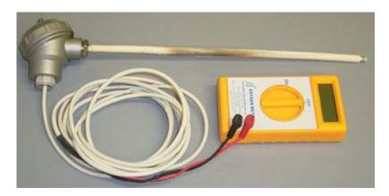
An oxygen probe works by comparing the oxygen level in the kiln with the oxygen level inside the alumina tube. This is why the air inside the tube must always be renewed. If the temperature of the zirconia tip is over about 700 °C, it produces an electrical voltage. The less oxygen in the kiln, the bigger the electrical voltage, so the voltage can be used as a guide to the oxygen level.
