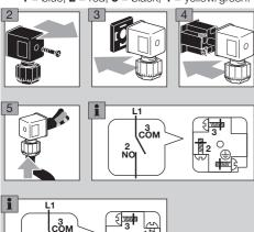
⊳ Plug insert can be rotated in 90° steps.
