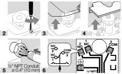
→ DG..FT, DG..NT: the NO-to-COM connection is interrupted if the pressure drops (contacts 3 and 2 open). DG..T, DG..HT: the NC-to-COM connection is interrupted if the pressure rises (contacts 3 and 1 open).
