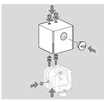
8.5 Cover IP 65 with pressure equalization element
