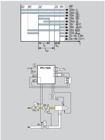
Parameter 30 = 0: The air valve opens if it is activated externally by input 10a.
