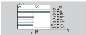
If the flame fails during operation, the valve outputs are disconnected within the safety time  $t_{SB}$ .
