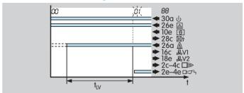
An extraneous signal is an incorrect signal which is detected as a flame signal out of sequence. If the PFU 760 notices such an extraneous signal during the flame simulation check, it starts the flame simulation delay time  $t_{\rm LV}$ . If the extraneous signal is discontinued during this period, the burner can start up. Otherwise, a fault lock-out occurs.  $\boxed{\Box I}$  blinks on the display.
