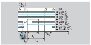
If the PFU detects a flame failure after a minimum operating time of 2 s, the valves are closed and the operation signalling contact is opened within time  $t_{SB}$ .
