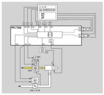
A switchable gas solenoid valve V2 can be activated with the PFU..L. If Parameter 26 is set to 1, gas valve V2 can be activated synchronously with the air valve during operation via the input for the external activation of the air valve (terminals 10a/12a).
