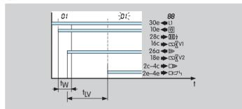
An extraneous signal (flame simulation) is a flame signal that is detected, although there should be no flame according to the program sequence. If such an extraneous signal is detected, the flame simulation delay time  $t_{LV}$  starts to elapse. If the flame simulation is discontinued during the flame simulation delay time  $t_{LV}$ , start-up can be initiated or operation continued. Otherwise, a fault lock-out occurs.
