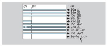
When High temperature mode is ended, the burner remains in operation and the PFU performs flame control again (recommended in the case of ionization control or UV control with UVD).
