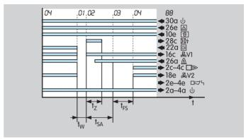
When High temperature mode is ended, the PFU switches off the burner and restarts with flame simulation check (recommended in the case of UV control with UVS).
