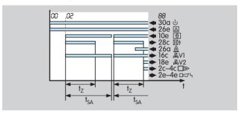
If several start-up attempts are set and if the PFU detects a flame failure during start-up, it closes valve V1 after the safety time  $t_{SA}$  has expired and attempts to start up again. After the last programmed start-up attempt has been completed, the burner control unit conducts a fault lock-out. The display blinks and shows the cause of the fault.
