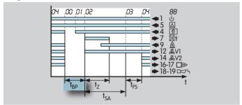
An immediate restart of the main burner after a controlled shut-down, a start-up attempt, restart, cooling or purging is prevented by the pause time. The pause time starts when the air valve is switched off. If a start-up signal (9) is applied before expiry of this time, the start-up is delayed until the end of the pause time.
