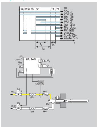
Parameter 30 = 0: The air valve opens if it is activated externally via input 10a.
