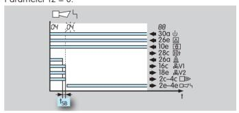
After a fault lock-out, the burner control unit can be reset, either with the button on the front panel or using an external button. Several burner control units can be reset in parallel using the external button.
