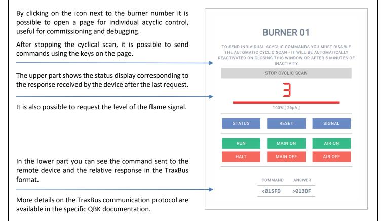
In the main page of the webserver the flame signal will be reported only for the burners that have this option enabled, while it is always possible to view it on the individual control page of the remote device.
