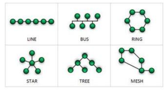
TraxBus<sup>™</sup> lines can be wired in any form: star, ring, line or mixed but signal line must be wired separately from power lines. Do not use shielded cables. Do not use multicore cables or limit the usage to short stubs.
