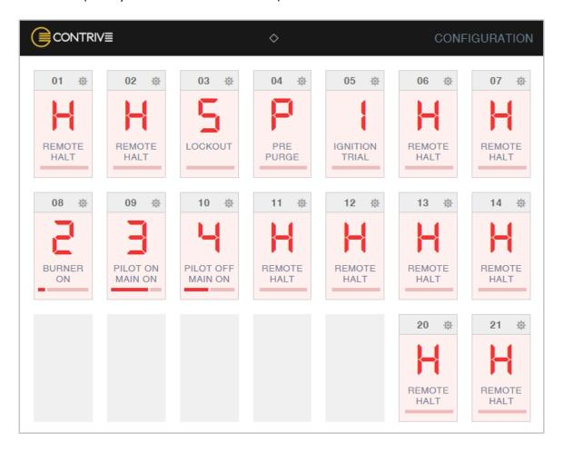
On this page there is a panel that shows status and flame signal of the burners installed, each with its own numbering. This status is updated cyclically and corresponds to the information made available on the PROFINET-IO side.
