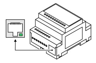
THE GREEN LED ON THE RJ45 CONNECTOR IS A COMBINED LINK AND ACTIVITY INDICATOR:
