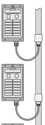
Burner controller having address 21 is controlled by input contact 2: close to start and open to stop the burner, behavior similar to a thermostat.
