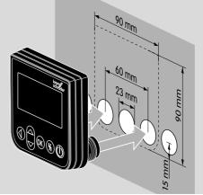
**3** Screw the nuts on to the threaded adapters so that the OCU is firmly attached to the door.
