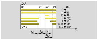
If the IFD detects a flame failure after a minimum operating time of 2 s, the valves are closed and the operation signal-ling contact (terminals 13 and 14) is opened within time  $t_{\rm SB}$ .
