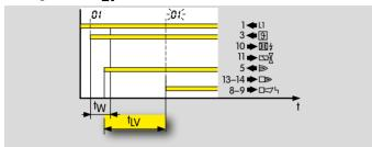
Flame simulation is an incorrect flame signal. If flame simulation is detected during start-up, the flame simulation delay time  $t_{LV}$  (max. 25 s) starts to elapse. If the flame simulation is discontinued during the flame simulation delay time  $t_{LV}$ , start-up can be initiated or operation continued. Otherwise, a fault lock-out occurs.
