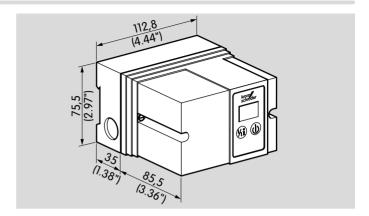
The housing is made of impact-resistant plastic. The upper section containing the detection circuitry is a push connection fit into the lower section. The connection terminals, grounding strip and neutral bus are located in the lower section. The upper section of the housing is attached to the lower section using two screws.
