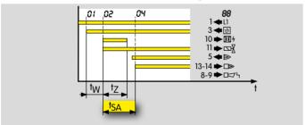
This refers to the period of time between switching on and switching off of the gas valve V1, when no flame signal is detected. The safety time on start-up  $t_{SA}$  (3, 5 or 10 s) is the
