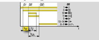
Once the start-up signal  $\vartheta$  has been applied, the waiting time  $t_W$  starts to elapse. During this time, a self-test is conducted to detect errors in internal and external circuit components. If no malfunction is detected, the burner will start up.
