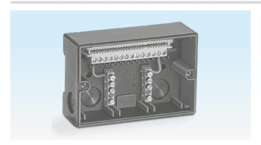
The lower section can either be snapped onto a DIN rail or secured with two M5 screws. In order to obtain enclosure IP 54, two sealing washers must be placed beneath the M5 screws.
