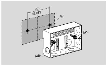
The housing has 6 knock-out holes for M16 plastic cable glands.
