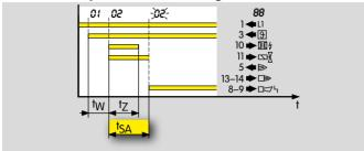
If, after a successful burner start, the automatic burner control unit does not detect a flame signal during the safety time on start-up  $t_{SA}$ , a fault lock-out will occur (fault signalling contact between terminals 8 and 9 closes). During the entire safety time on start-up  $t_{SA}$ , the gas valve V1 is open. The display blinks and indicates  $\mathcal{B}\mathcal{H}$ .
