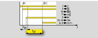
If flame simulation is signalled during start-up, the flame simulation delay time  $t_{LV}$  starts to elapse. If the flame simulation is discontinued during the flame simulation delay time  $t_{LV}$  (max. 25 s), the burner will start up. Otherwise, a fault lock-out occurs. The display blinks and indicates  $\mathfrak{U}$ .
