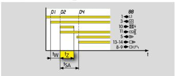
If no malfunction is detected during the waiting time  $t_W$ , the ignition time  $t_Z$  then starts to elapse. Voltage is supplied to the gas valve V1 and the ignition transformer and the burner is ignited. The duration of the ignition time is either 2, 3 or 6 s, see page 27 (Technical data).
