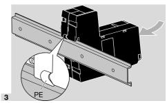
→ Ensure there is a good PE (ground) wire connection between the DIN rail and the BCM's PE contact.
