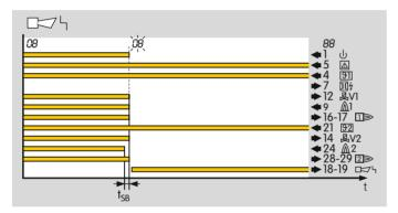
After a flame failure, the burner control unit performs a fault lock-out within the safety time during operation  $t_{SB}$ . This involves disconnecting the power from the gas valves and the ignition transformer. The fault signalling contact closes, the display blinks and shows the current program status, see table on page 27 (Program status and fault messages).
