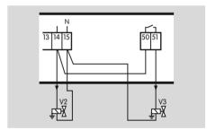
The opposite application describes a two-stage-controlled burner without a pneumatic air/gas ratio control system. The third gas valve (V3) and the air valve are activated simultaneously. During purging/cooling, the gas valve (V3) is not activated
