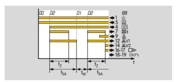
If several start-up attempts are set at the works and if the BCU detects a flame failure during start-up, it closes valve V1 after the safety time  $t_{SA1}$  has expired and attempts to start up again. After the last programmed start-up attempt has been completed, the burner control unit conducts a fault lock-out. The display blinks and shows the cause of the fault
