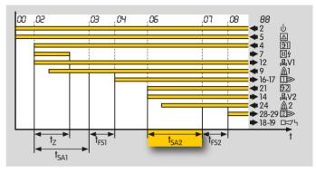
This indicates the safety time on start-up  $t_{\text{SA2}}$  for the main burner.
