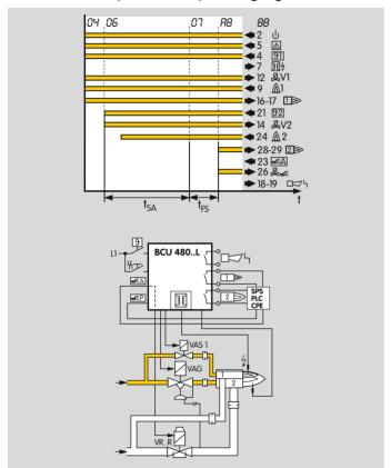
Parameter 30 = 3: The air valve opens simultaneously with the operating signal.
