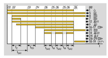
If several start-up attempts are set at the works and if the BCU does not detect a flame signal during start-up, it closes valve V2 after the safety time  $t_{SA2}$  has expired and attempts to start up again. After the last programmed start-up attempt has been completed, the burner control unit conducts a fault lock-out. The display blinks and shows the cause of the fault.
