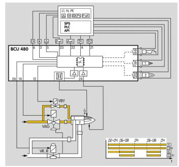
The pause time has an effect on the behaviour of the main burner only. Reason: the pilot burner is only used in single-stage operation.
