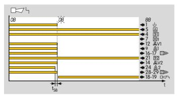
If the flame fails during operation, the valve outputs are disconnected within the safety time  $t_{SB}$ .
