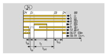
If the BCU detects a flame failure after a minimum operating time of 2 s, the valves are closed and the operation signalling contact is opened within time  $t_{SB}$ .
