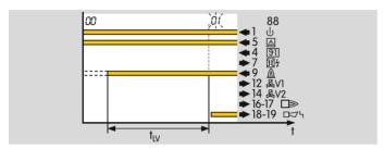
If the BCU notices an extraneous signal during the flame simulation check, it starts the flame simulation delay time  $t_{LV}$  (25 s). If the extraneous signal is discontinued during this period, the burner can start up. Otherwise, a fault lock-out occurs.  $\boxed{I}$  blinks on the display if an extraneous signal is detected by the pilot burner and  $\boxed{5}$  blinks if an extraneous signal is detected by the main burner.
