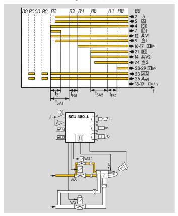
Parameter 30 = 0: The air valve opens if it is activated externally via input 23.
