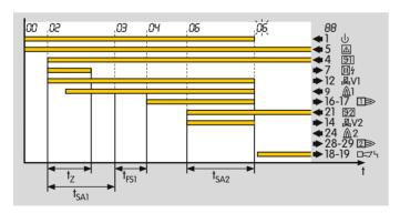
If no flame forms during the start-up of the main burner, a fault lock-out is performed after expiry of time  $t_{SA2}$ . The display blinks and shows the cause of the fault.
