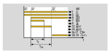
If no flame forms during start-up, a fault lock-out is performed after expiry of time  $t_{SA}$ . The display blinks and shows the cause of the fault
