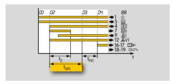
This indicates the safety time on start-up  $t_{\text{SA1}}$  for the pilot burner.
