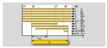
In the case of pilot/main burner monitoring, the minimum burner on time only has an effect on the behaviour of the main burner. The minimum burner on time for the pilot burner is limited to the safety time on startup ( $t_{S\Delta}$ ).
