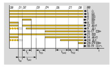
The BCU switches off the burner once the DI input has been disconnected from the electrical power supply and restarts with flame simulation check (recommended in the case of UV control with UVS).
