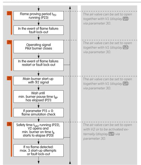
The BCU coordinates the correct program run for the pilot and main burners. The main burner can be started via the signal input "Start-up signal  $\vartheta$ 2" (terminal 21) if required.
