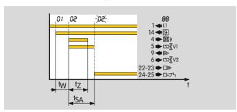
Once the start-up signal  $\vartheta$  has been applied, the waiting time  $t_W$  starts to elapse. During this time, a self-test is conducted to detect errors in internal and external circuit components. If no malfunction is detected, the burner will start up.
