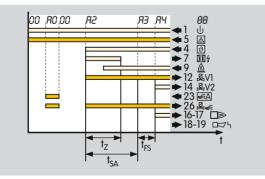
Parameter 30 = 1: The air valve opens simultaneously with valve V1.
