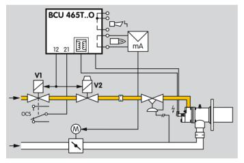
Parameter O9 = 1: A signal is sent to the BCU via the position indicator on the gas solenoid valve V1 stating whether the valve is closed or open. In standby, the switch must be closed. During start-up and operation, the switch must be open. This ensures that valve V1 is open or closed.
