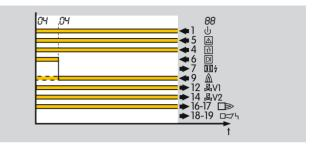
The burner remains in operation and the BCU performs flame control again (recommended in the case of ionization control or UV control with UVD).
