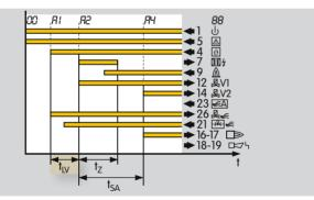
After the start-up signal  $(\vartheta)$  has been applied and after the flame simulation check and "no flow" state check have been conducted successfully, the air valve is opened. Start-up of the burner commences as usual with no interruption of the air after expiry of the programmable pre-ventilation time  $t_{VL}$ . (Parameter setting for this example sequence: P15 = 1, P23 = 0, P30 = 1, P37 > 0), see page 41 (Parameters). The gas valve does not open until the pressure switch has switched.
