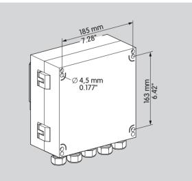
Die-cast aluminium housing with plug-in terminal blocks and plug-in M20 cable glands or (16-pin) plug connector for input signals and optionally pre-assembled cables for output signals.
