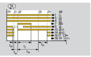
If the BCU detects an installation fault (flame failure or failure of air flow) after a minimum operating time of 2 s, the valves are closed and the operation signalling contact is opened within time  $t_{SB}$ .
