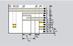
Parameter 30 = 2: The air valve opens simultaneously with valve V2.
