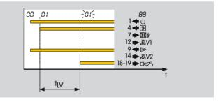
The flame simulation check of the burner is active until valve V1 is enabled.
