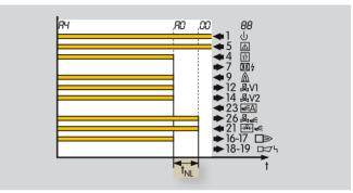
The air valve remains open for the programmed time after the start-up signal ( $\vartheta$ ) has been deactivated. The burner control unit closes the air valve after expiry of the post-ventilation time  $t_{NL}$ .
