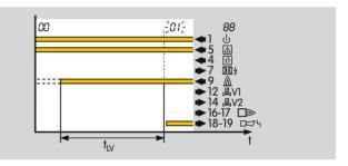
Flame simulation check on start-up (parameter 15 = 0):
