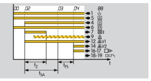
If the temperature in the furnace chamber drops below 750°C, the DI input must be disconnected from the electrical power supply and the furnace must then be operated with flame control.
