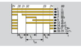
An immediate restart of the burner after a controlled shut-down is prevented by the pause time. The pause time starts when the burner is switched off. If a start-up signal ( $\vartheta$ ) is applied before expiry of this time, start-up is delayed until the end of the pause time.
