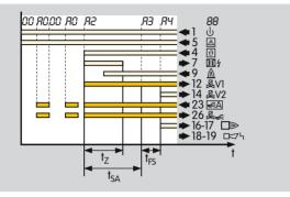
Parameter 30 = 0: The air valve opens if it is activated externally by input 23.
