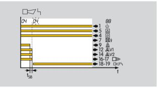
After an installation fault (flame failure or failure of air flow), the burner control unit performs a fault lockout within the safety time during operation  $t_{SB}$ . This involves disconnecting the power from the gas valves and, if applicable, the ignition transformer. The fault signalling contact closes, the display blinks and shows the current program status, see table on page 39 (Program status and fault messages).
