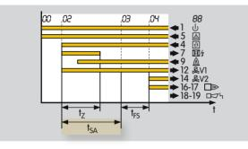
This indicates the safety time on start-up  $\ensuremath{t_{\text{SA}}}$  for the burner.
