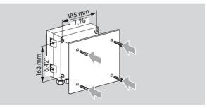
Screw on the closed unit to the rear with 4 self-tapping screws (enclosed).
