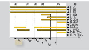
With this function, the combustion chamber can be purged after a safety shut-down in compliance with standards, especially on radiant tube burners. This task is not implemented by a central control system but by the BCU 465. See also parameters 40 and 41.
