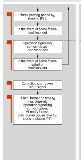
The air valve can also be set to open with V2 or to be activated externally (display 🖽) via parameter 30. This completes start-up. An adjustable min. burner on time  $t_B$  ensures that the burner burns for a defined period even if the start-up signal ( $\vartheta$ ) is switched off beforehand.
