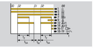
If several start-up attempts are set at the works and if the BCU detects an installation fault during start-up, it closes valve V1 after the safety time  $t_{SA}$  has expired and attempts to start up again. After the last programmed start-up attempt has been completed, the burner control unit conducts a fault lock-out. The display blinks and shows the cause of the fault.
