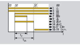
If no flame forms or, in the case of BCU 465, if the air flow fails during start-up, a fault lock-out is performed after expiry of time  $t_{SA}$ . The display blinks and shows the cause of the fault.
