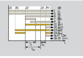
Parameter 30 = 0: The air valve opens if it is activated externally by input 23.
