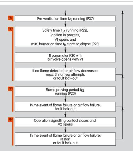
If both flame and air flow are detected during the safety time  $t_{SA}$ , the flame proving period  $t_{FS}$  starts after this safety time has elapsed. Valve V2 opens and the operation signalling contact between terminals 16 and 17 closes. This completes start-up. An adjustable min. burner on time  $t_B$  ensures that the burner burns for a defined period even if the start-up signal ( $\vartheta$ ) is switched off beforehand.
