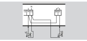
The following application describes a two-stage-controlled burner without a pneumatic air/gas ratio control system. V2 and the air valve are activated simultaneously. However, V2 may not be activated during purging.
