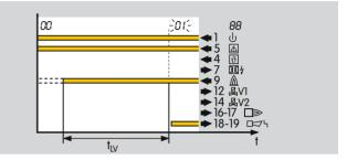
An extraneous signal (flame simulation) is a flame signal that is detected, although there should be no flame according to the program sequence. If such an extraneous signal is detected, the flame simulation delay time  $t_{LV}$  starts to elapse. If the flame simulation is discontinued during the flame simulation delay time  $t_{LV}$ , start-up can be initiated or operation continued. Otherwise, a fault lock-out occurs.
