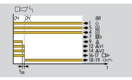
If the flame fails during operation, the valve outputs are disconnected within the safety time  $t_{\mbox{SB}}.$
