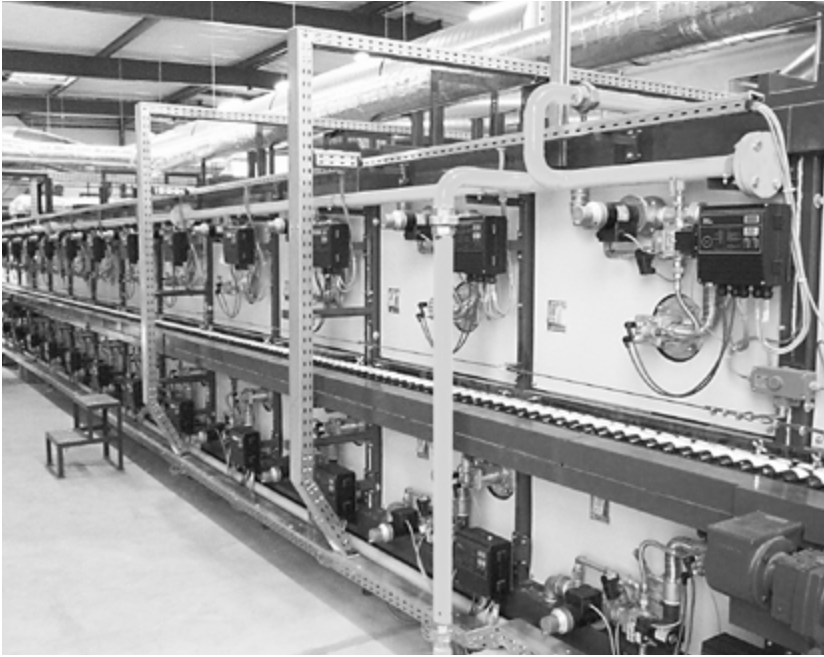
Roller hearth kiln in the ceramics industry
