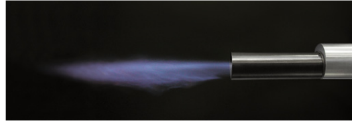
Flame of the ZKIH during natural gas operation in the open air
