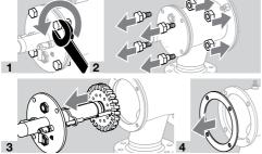
**5** Place the burner insert in such a way that the insulators are protected against damage.
