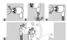
6 Connect the PE wire for burner ground to the burner insert. In the case of single-electrode operation, route the PE wire from the burner insert directly to the terminal on the automatic burner control unit.
