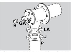
→ The nozzle set with NPT thread is required for integrated pilots, see page 12 (9.3 Nozzle set).
