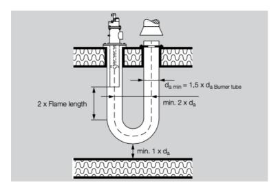
When using the burner in radiant tubes or flame tubes, the extended burner tube (attachment tube) acts as the combustion chamber. Burners for this field of application are supplied with purge air bore holes for optimal flame stability.
