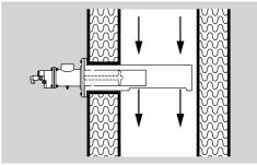
→ At flow velocities of > 15 m/s, the flame tube FPT is used to protect the flame from being cooled.
