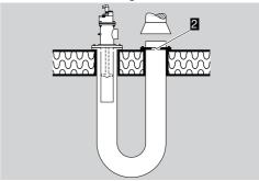
→ Reduce the outlet diameter of the radiant tube using an orifice 2 to the point where a pressure loss of approx. 10 mbar occurs at the burner's rated capacity.
