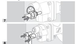
→ Turning the spark plug makes it easier to feed the electrode into the burner insert.
