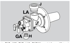
→ BIO 125, BIO 140, BIOW: weld flange K to air pipe P for air connection LA and use NPT thread adapter H for gas connection GA.
