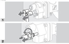
→ Ensure that the electrode length does not change.3 Remove dirt from electrodes or insulators.
