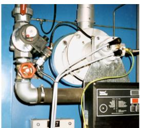
Direct heating of a roller hearth furnace.
