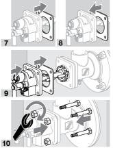
→ Tighten burner insert in a crosswise fashion: BIC(A) 50 to 100 with max. 15 Nm (11 lb ft), BIC 125 to 140 with max. 30 Nm (22 lb ft).
