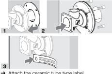
→ Attach the ceramic tube type label.
