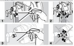
→ Avoid condensation due to the furnace atmosphere entering the burner body. While the burner is switched off, at furnace temperatures above 500°C (932°F), it must be cooled with a low air volume – see page 11 (6.6 Cooling air).
