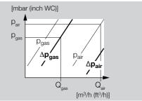
2 p1: gas pressure upstream of the measuring orifice,p2: gas pressure downstream of the measuring orifice. Measuring range: select approx. 15 mbar.
