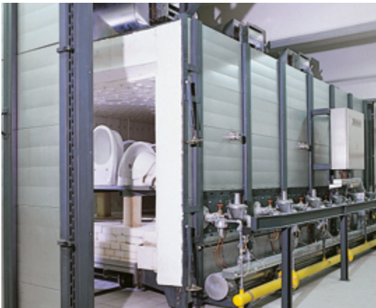
Ceramics kiln with temperature control via impulse system
