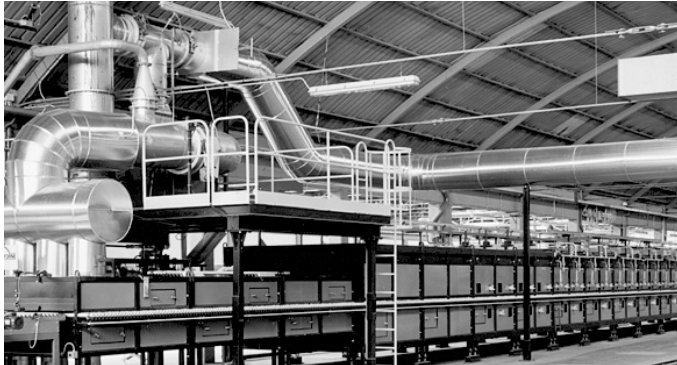
Roller hearth kiln in the ceramics industry
