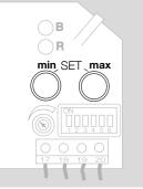
→ Calibration is completed when the blue LED is lit continuously and the red LED goes out.
