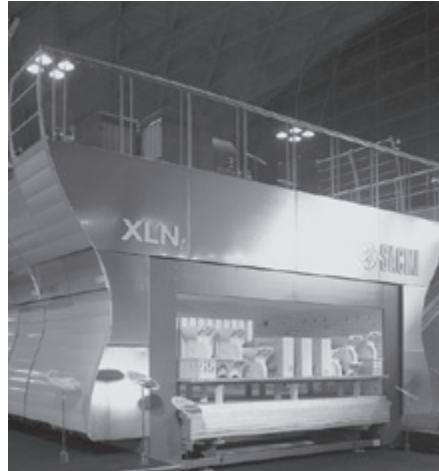
Roller hearth furnace
