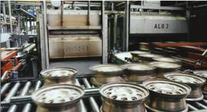
Aluminium industry: curing oven for wheel rims
