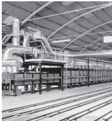
Roller hearth kiln in the ceramics industry
