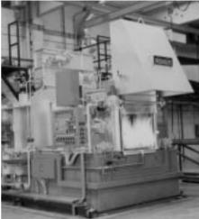
For safeguarding and controlling atmospheric burners, e.g. excess gas burners, flame curtains and one-stage burners, in addition to preheating burners.
