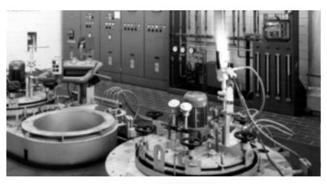
For safeguarding and controlling onestage atmospheric burners with pilot burner.
