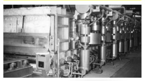
For safeguarding and controlling steplessly and stage-controlled burners with pneumatic link between gas and air, e.g. recuperative burners.
