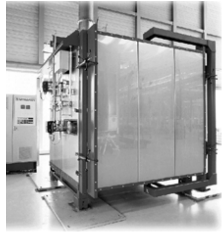
Chamber kiln for intermittent operation
