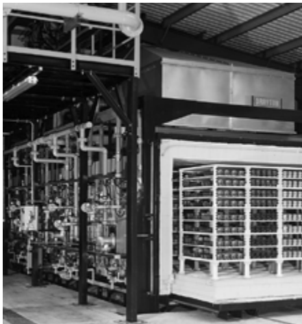
Intermittent shuttle kiln in the fine ceramics industry
