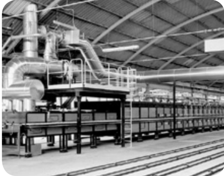
Roller hearth kiln in the ceramics industry
